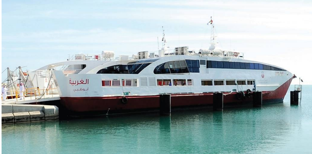
Photo 7-3: Typical Monopile Berthing Dolphins
